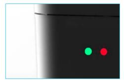
If the internet link is lost, the box will show blue/purple on the left LED. The box will try to reconnect itself. If the test is done (right LED is solid green), it is safe to turn off the box. The NudgeBox will automatically resend the previous test results before allowing users to start any new test.
