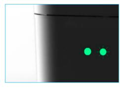
ix. When the test is complete both LEDs will show steady Green.
